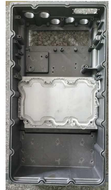
Friction welding of cavity and heat sink
